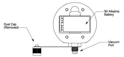
**Rear View (Battery Cover Removed)**
